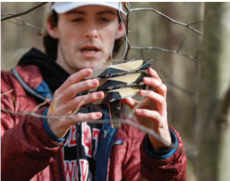
Luke Davies, '25, hangs a homemade shield containing a Lascar temperature and humidity data logger on a tree.
